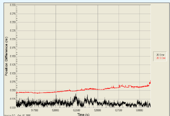
Figure 5: SMART-V1G Typical RT-20 Steady State (Horizontal)
